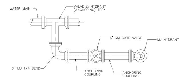
\* ALTERNATE: MJ TEE AND ANCHORING ELBOW
