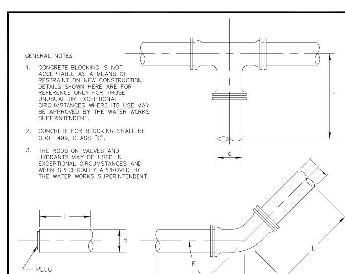
L = REQUIRED LENGTH OF RESTRAINED JOINTS
