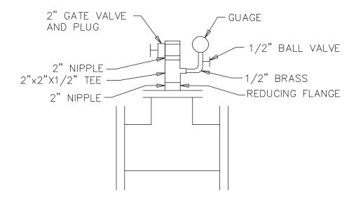
TEST ASSEMBLY DETAIL
